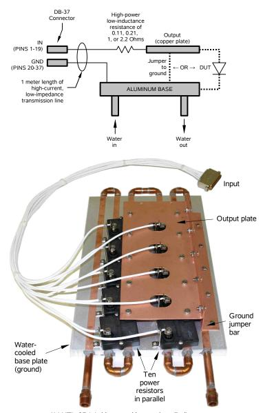
AV-HTL-0R1 (with ground jumper installed)
